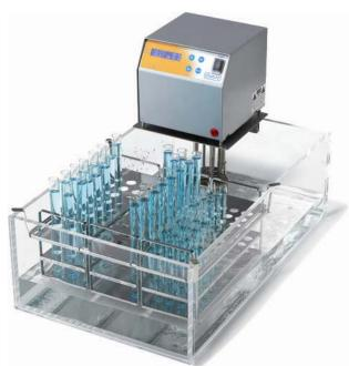
Transparent bath with digital immersion thermostat, controlled by microprocessor.
