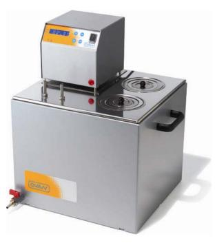
**Recirculating digital** bath with immersion thermostat, controlled by microprocessor.
