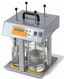
Digital portable flocculator controlled by microprocessor.
