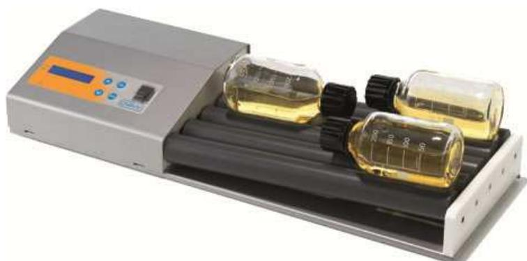
Digital rotary and oscillating mixer with rollers, controlled by microprocessor.
