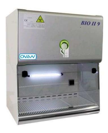
The laminar flow (Class 100FS 209E,ISO 5) sweeps the work space and protects the product. The air flow is completely recycled through the perforated grills around the work surface and the operator protection is made by air streaming in front of the work surface : about 30% of the air flow is thrown through an Hepa filter
