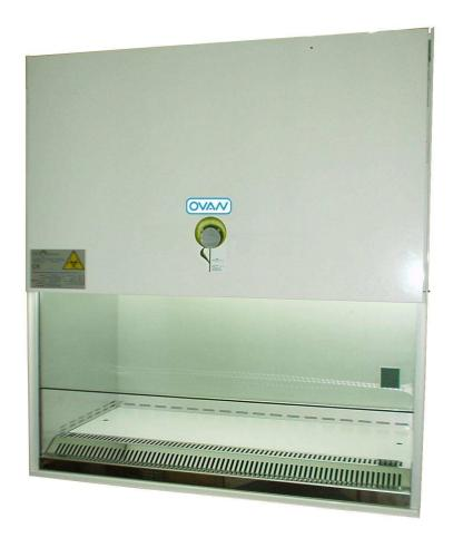
The laminar flow, Class 100FS 209, IS BLOWING THROUGH Absolute filter in the work volume insuring manipulation safety.
