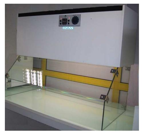
Filtration is performed thanks to activated active carbon filter, responsible to absorve all gases and vapours present in the air flow going through.
