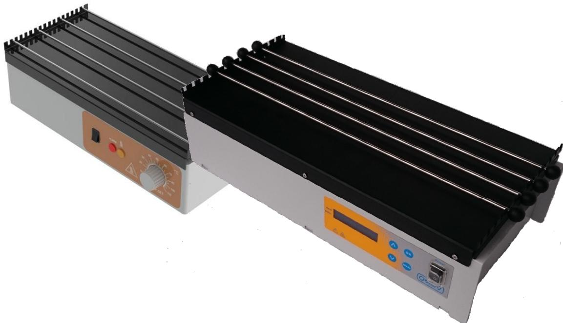
Slide Drying Units used in the preparation of microscope slides at preparation step.
