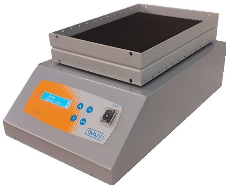
Digital orbital-vibrating shaker, controlled by microprocessor
