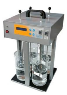
**Digital portable** flocculator controlled by microprocessor.
